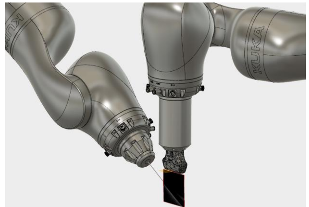
Figure. 1. CAD model of the two robots with the mounts for the needle and US transducer and shown with the US image overlaid.
