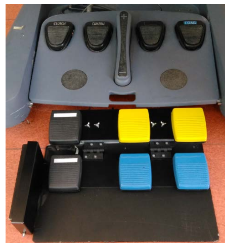
Figure 1 Photo of the supplement foot pedals tray and original DVRK foot pedals platform. The additional tray replicating the same pedals configuration used in recent da Vinci surgical system.
